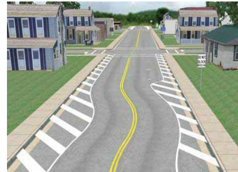
TEMPORARY CHICANES Temporary installations may be used prior to permanent installation. Temporary installations can be created through paint, temporary curbs, giant flower pots, or other creative uses. Photo credit: FHWA
