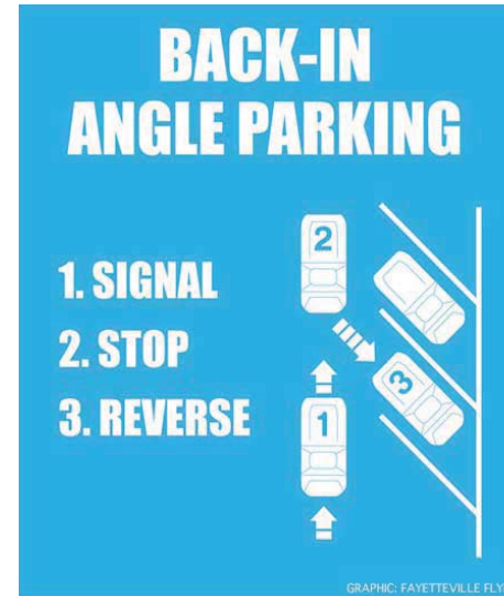
BACK-IN ANGLE PARKING Back-in angle parking increases visibility of cyclists for drivers pulling out of parking spaces. Photo credit: http://walkbikerjerry.blogspot.org
