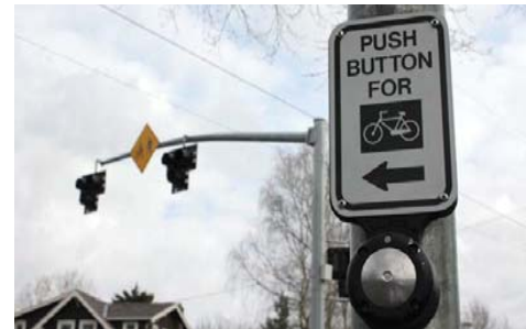
PUSH BUTTONS Enable cyclists to trigger signals, but requires them to dismount. Photo credit: NACTO
