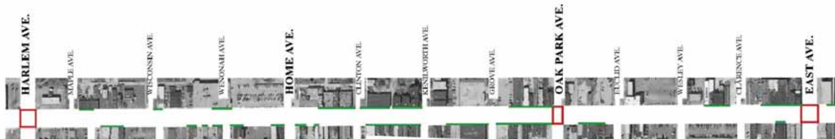
This PedZone SM diagram illustrates the lack of pedestrian continuity throughout the existing corridor. Note that the green bars indicating a rewarding pedestrian experience have significant breaks signalling a lack of continuity. The red bars indicate the existing crosswalks, illustrating their infrequency throughout the corridor.
